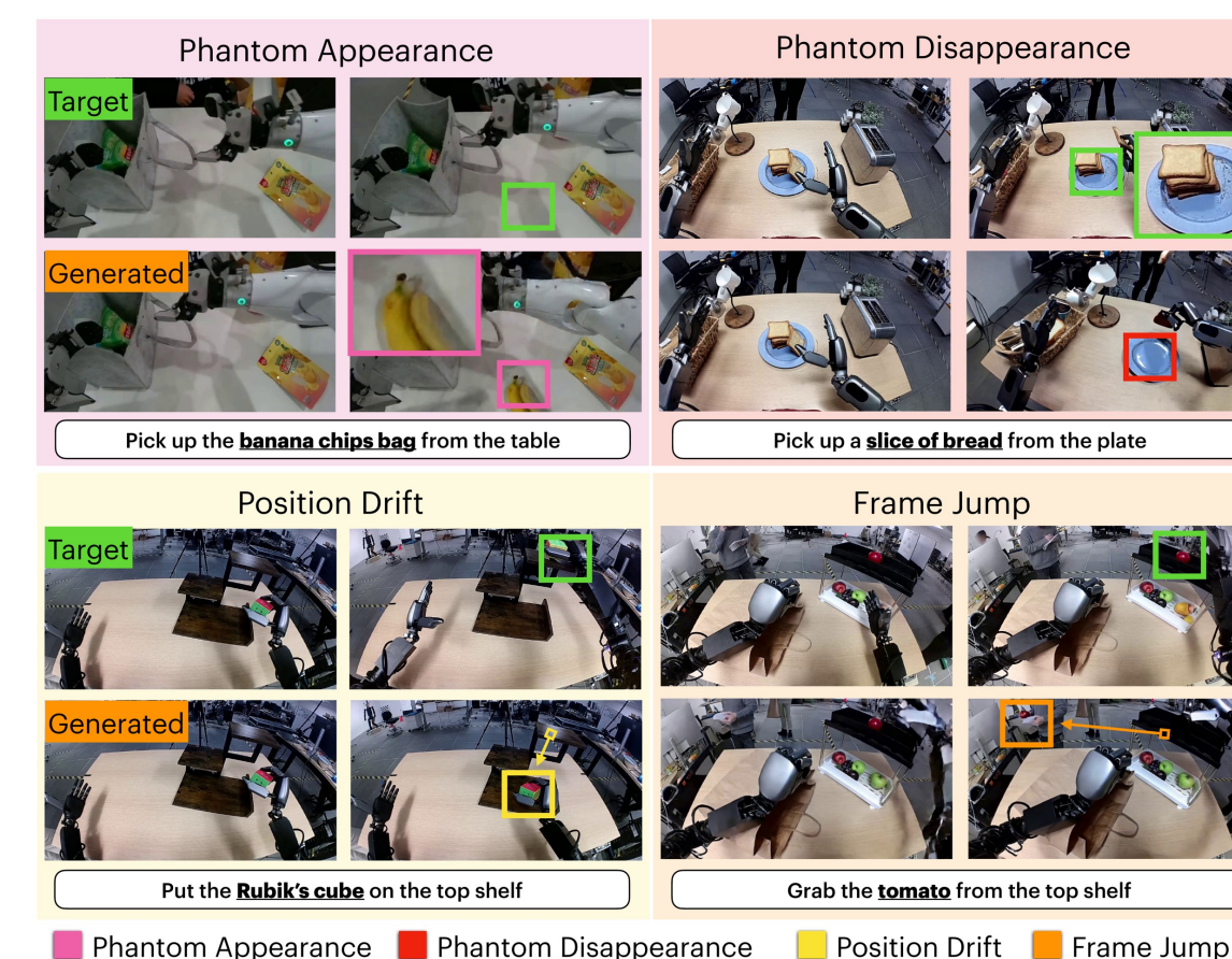
Fig. 2b · Failure modes. Real target vs. generated rollouts
